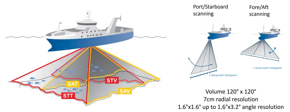
15 A multi-usage multibeam sonar for hydrography and robotics applications
