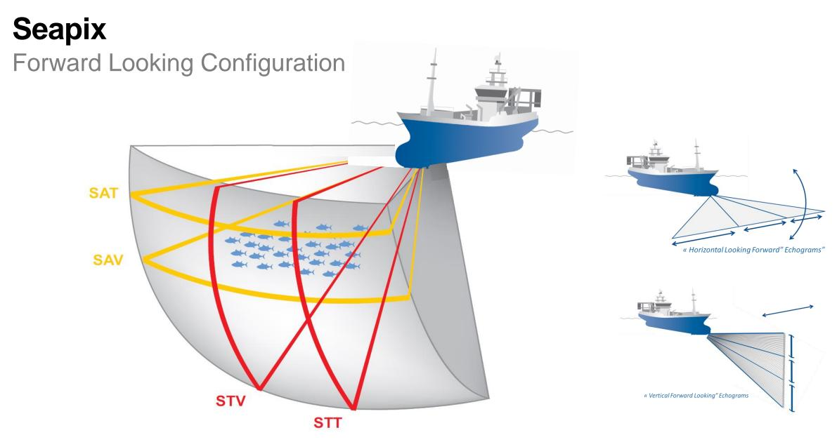
16 A multi-usage multibeam sonar for hydrography and robotics applications
