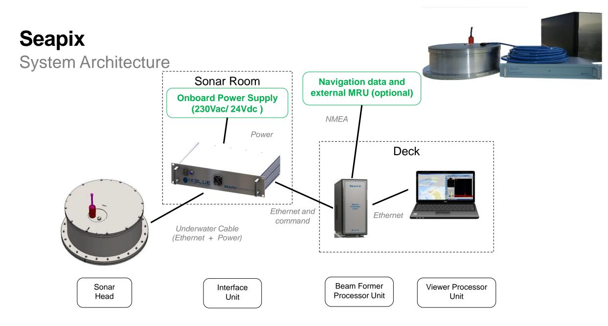
11 A multi-usage multibeam sonar for hydrography and robotics applications
